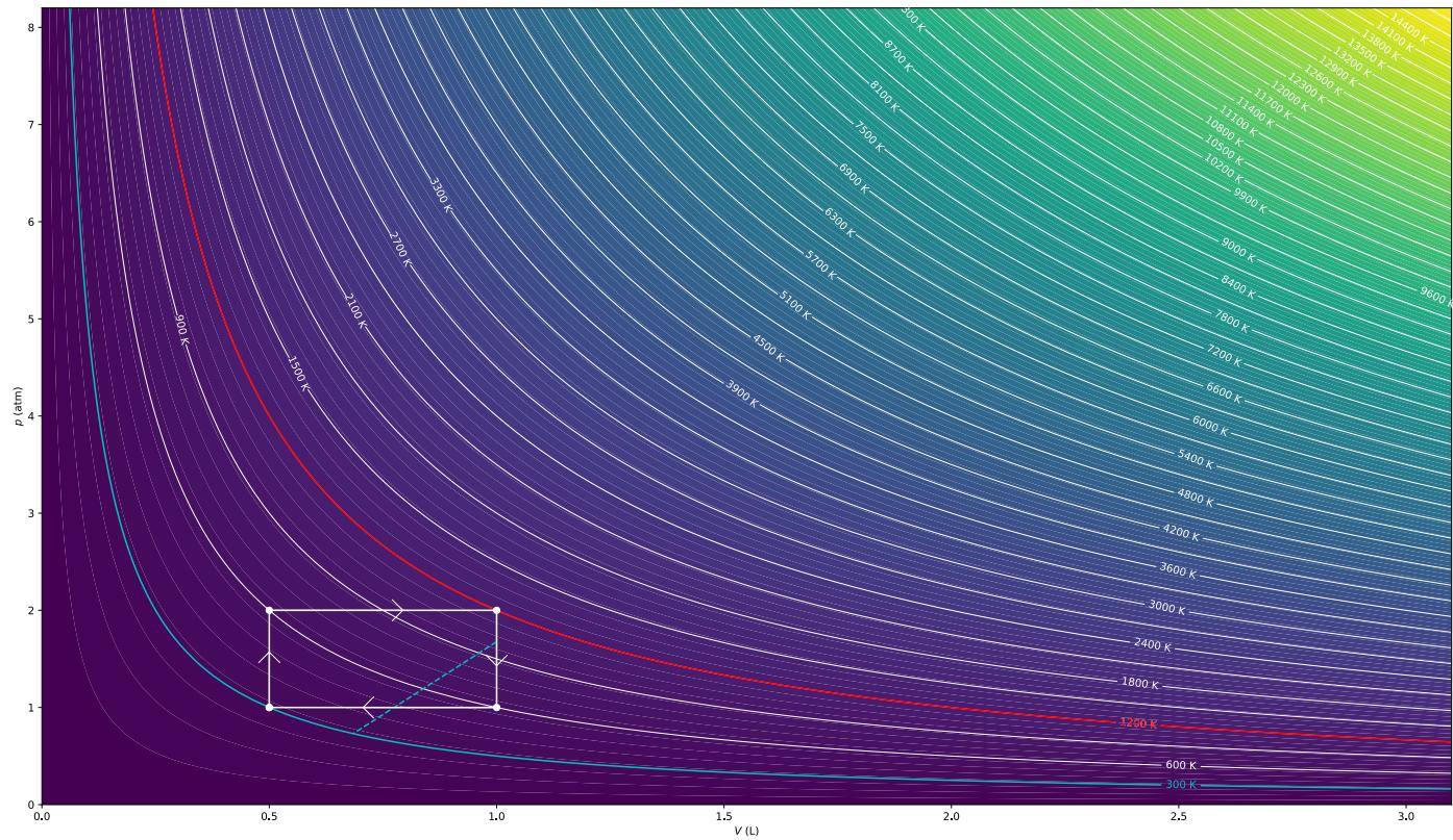
By the same token, on the third and fourth steps, when the gas is being cooled, the gas is heating its environment which is way cooler than the gas is, so again, we have a very irreversible process.
