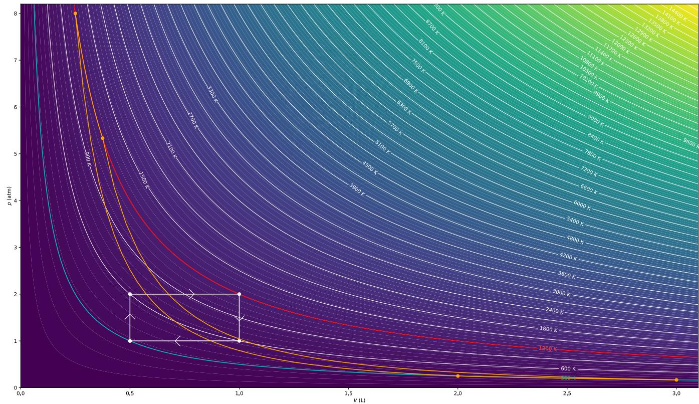
This diagram is hard to draw, and most humans draw it quite poorly. An easier way to draw the Carnot cycle would be with a  $TS$  diagram, with temperature on the horizontal axis and entropy on the vertical axis.
