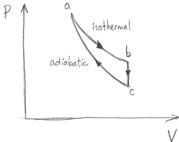
where the isothermal step occurs at constant temperature, and the adiabatic step has no energy transfer by heating.
