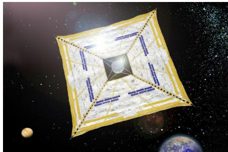
The first spacecraft using a solar sail for propulsion was launched in 2010. Its name is IKAROS. It has a square sail with dimensions 14 m x 14 m. Assume that the sail's mass is 2 kg and it reflects 100% of incident photons. When IKAROS is loaded with other equipment, the total mass of the vehicle is 10 kg. The sail is orientated to receive maximum light from the sun.
